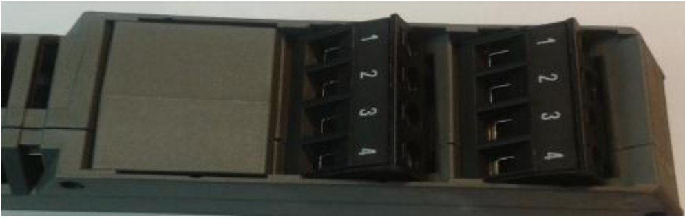
Terminals on the top side, with cover over the switch.
