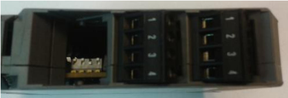
Terminals on the top side, with cover removed and switch accessible.
